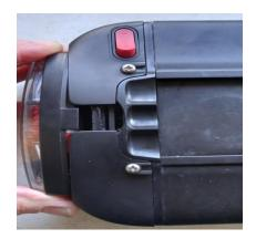
Remove the battery from the rear rack and turn it over.
